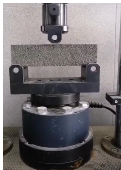
Figure 4. Determination of flexural strength of concrete samples
