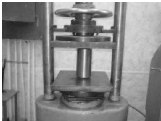
Figure 3. Compaction of the mixture on the press
