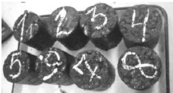
Figure 2. Appearance of remolded samples
