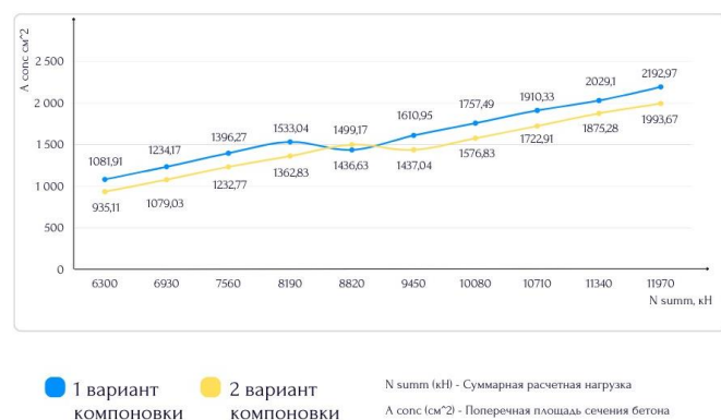
Figure 2. Graph of the dependence of the cross-sectional area of concrete on the total design load on the column
