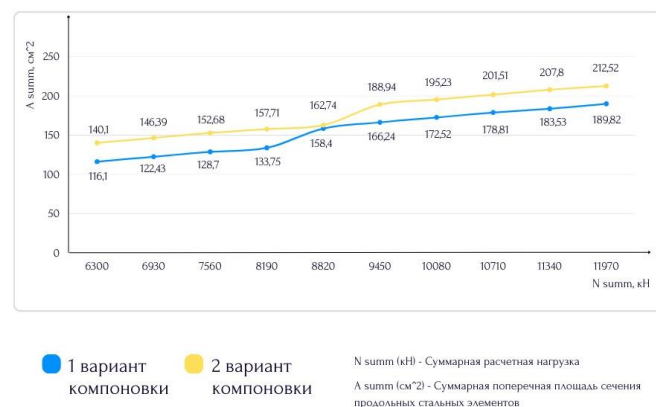
Figure 1. Graph of the dependence of the total cross-sectional area of longitudinal steel elements on the total design load on the column
