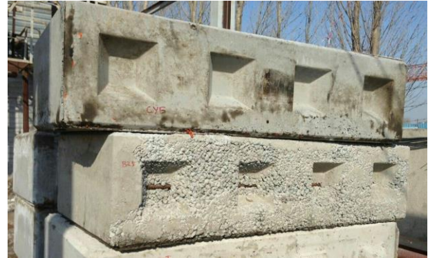
Figure 2. products made of secondary and ordinary cast concrete After facing
