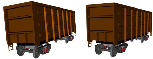
Figure 4. Forms of wagon oscillations: upper lateral roll – on the left, bouncing – on the right
